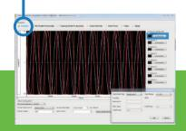
Quickly configure the signal acquisition settings, such as channel, range, single ended / differential inputs, sampling rate, memory size and trigger. No programming required.
